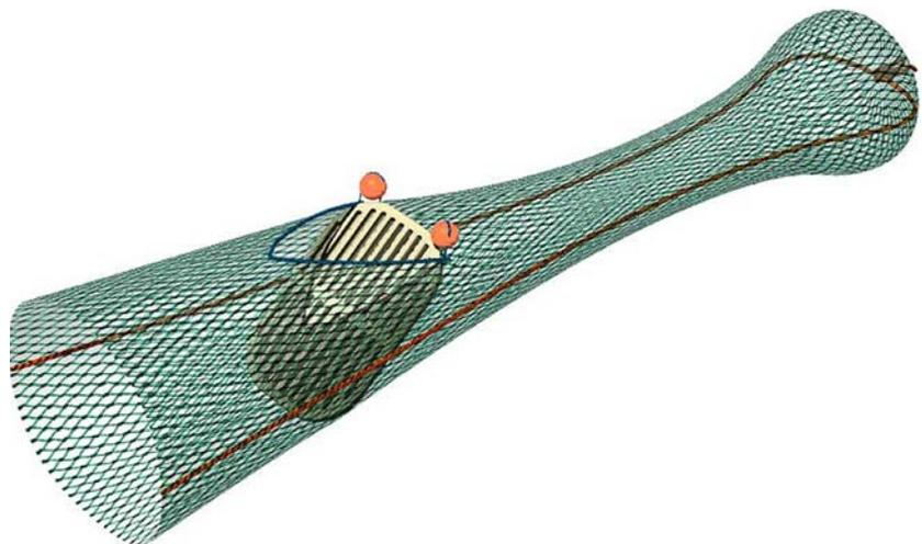
50 mm mesh separator panel positioned 75 cm above the bottom sheet. With this configuration, 94% of whiting and 96% of haddock were separated from 99% of *Nephrops* and 100% of cod (Main and Sangster 1982). Further trials have continued to demonstrate an effective separation of *Nephrops*, but when encountering larger numbers of whiting and haddock the level of separation is reduced (Hillis 1989; Sangster et al. 1990; Dunlin 1999).
