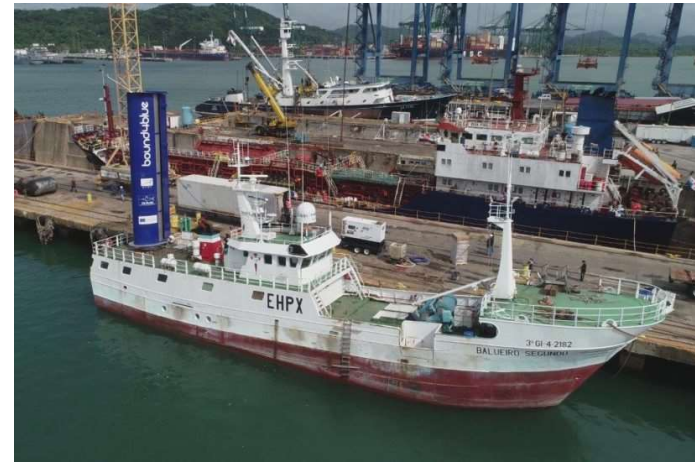
Balueiro Segundo with eSAIL® system, co-funded via EU Aspiring Wingsails project Vigo, Spain
