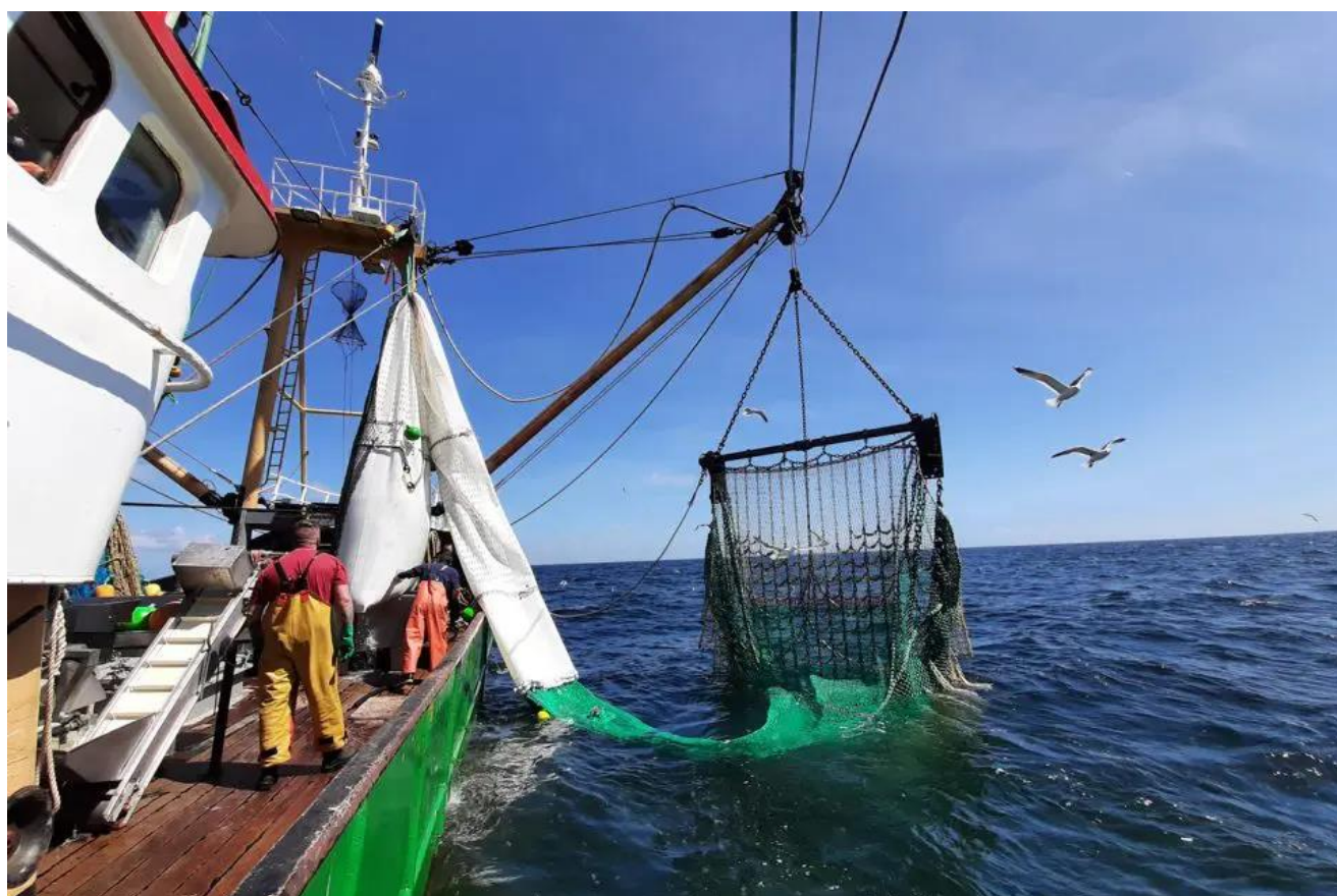
Figure 13: Hauling the cod-end of a net (picture source 'Globalseafood.org')
